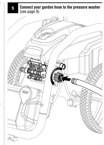
Completely uncoil garden hose or remove completely from reel to prevent kinks.
